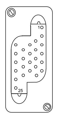
Figure 11 · Control signal connections
